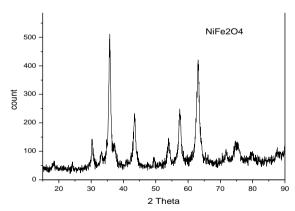
Figure 1. X-ray of Fe2NiO4 nanoparticle
