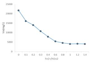
Figure 4. Impact of Fe2+ with peroxide on the disintegration of excess sludge
