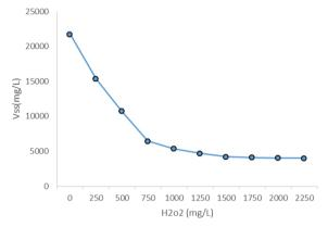
Figure 1. Impact of peroxide on the disintegration of excess sludge
